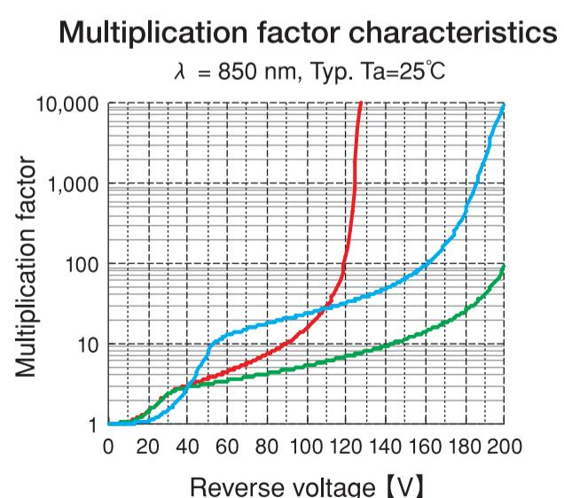
—— Low temperature coefficient    —— High speed    —— Low capacitance + Low dark current
