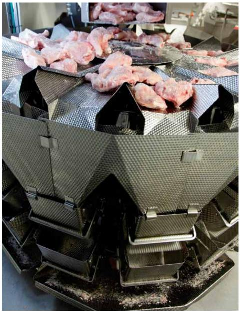
Even with this reject solution, the weigher is still able to operate at the required speeds, achieving – in tandem with the bagmaker - around 35 to 40 packs per minute on the chicken quarters, depending on bag size, while smaller and easier to handle pieces such as 900g packs of chicken fillets can be packed at around 50 bpm.
